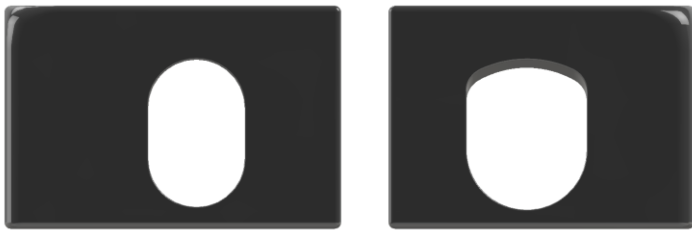
Fig. 5 Side slots on container corners
