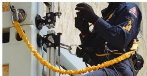
A suspension and fall arrest system using an anchor point at the top of the ladder and an optional corner anchor
