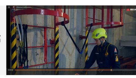
VRAPP at Height makes it possible to practice rigging anchor points and anchor point systems correctly.
