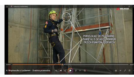
VRAPP at Height makes it possible to practice climbing on a step ladder with proper fall protection equipment and negotiating an edge.
