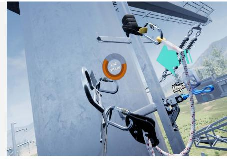
To perform this exercise, you will need a harness, a double fall arrest lanyard, a tape sling, a work positioning lanyard, and a fall arrest slider.
