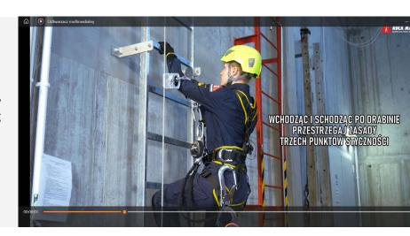
VRAPP at Height makes it possible to practice using the Tracker device as fall protection while climbing a chimney.
