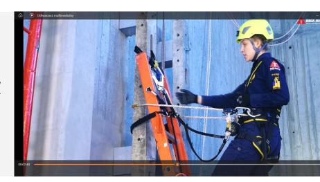
VRAPP at Height makes it possible to practice using a work positioning lanyard to set up an anchor system for work.
