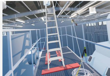
To perform this exercise, you will need a harness, an adjustable fall arrest lanyard, a sling, a pulley roll, and rope.
