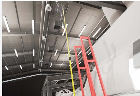
To perform this exercise, you will need a harness, an anchoring hook, a self-retracting lanyard, and a telescopic pole.
