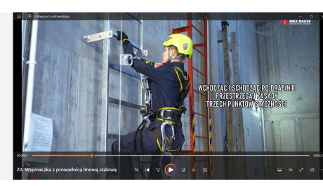
VRAPP at Height makes it possible to practice entering a roof using an external fixed ladder and a double fall arrest lanyard and setting up an anchor for suspension work.
